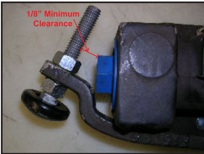
Figure 1 - ELX-B with Plastic Cap Nut. Minimum 1/8" clearance must exist at location indicated and throughout full sensor arm travel. Arm shown with brakes in release position.
